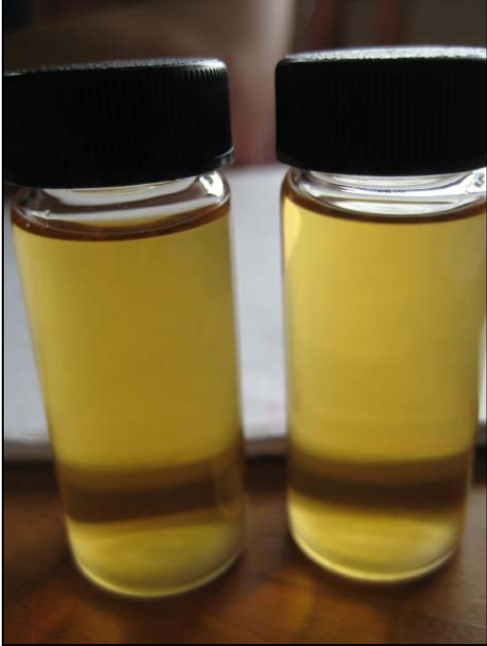
Figure 22: Pathoscreen Test at Start of Test (Left – Tap Water, Right – River Water)
