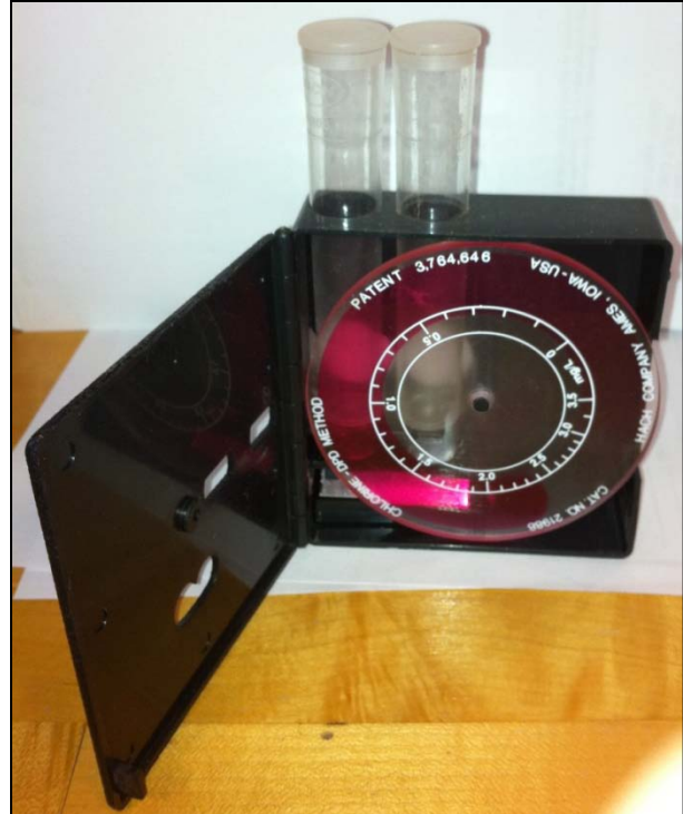
Figure 21: Open Color Wheel Device
