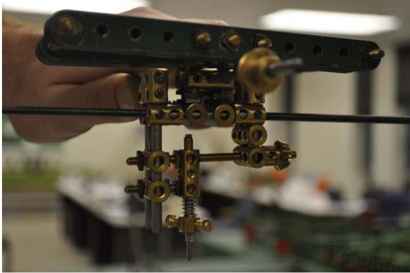
Figure 2.27. Side View of the Ordinate Carriage of the Output Table. The various couplings used in its construction and the spring loaded pen are shown. Also, green flat strips are screwed together and used to stabilize the carriage on the rails.
