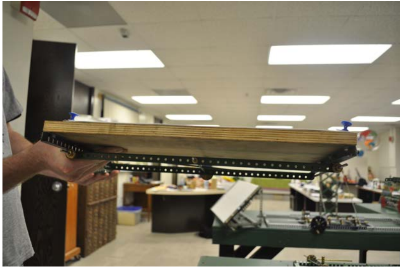
Figure 2.24. Side View of an Output Table Cart; its surface lies flat as opposed to the Input Table Cart.
