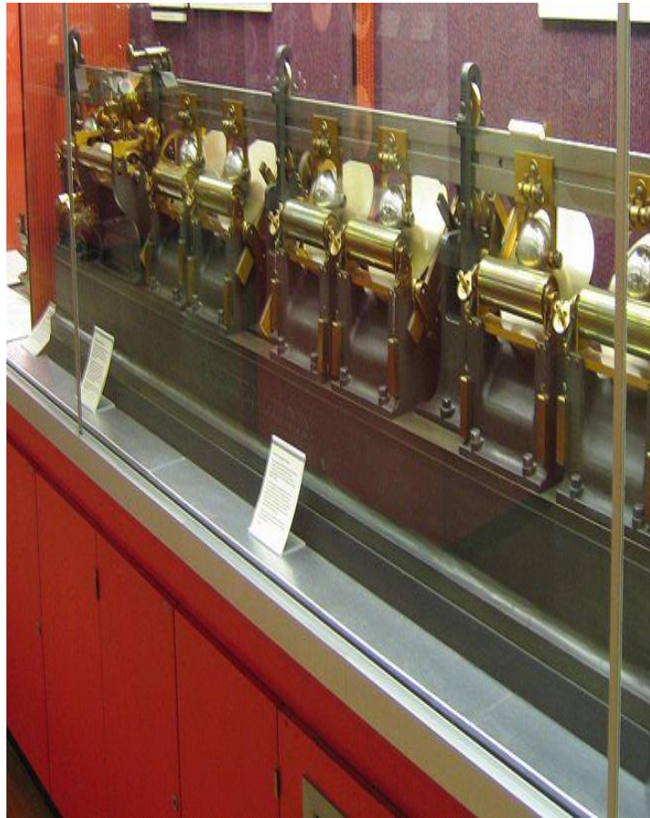
Figure 1.1. A picture of Thomson's integrating machine, Author: Andy Dingley; taken from his own work
