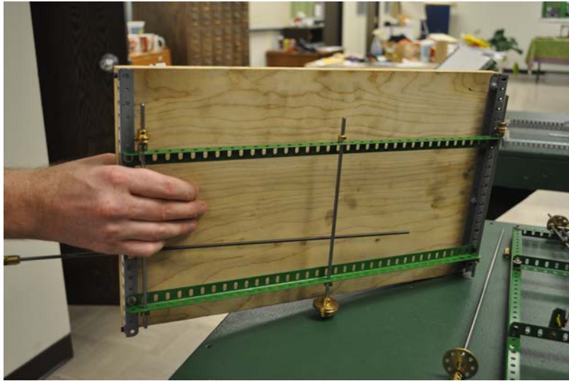
Figure 2.25. Under View of the Output Table Cart. The axial attachments for the wheels and the lead-screw driving rod are depicted.
