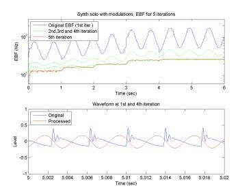
**Fig. 8.** (upper) EBF over 5 iterations of Multipass CoBE converging to the lowest frequency of the signal (the sample is the same shown in Fig. 3). (lower) Input waveform and waveform after 4 iterations of Multipass CoBE. The processed signal is suitable for ZCR pitch tracking algorithms.
