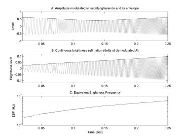
**Fig. 7.** The brightness value "B" of the sinusoidal input "A" can be turned into the frequency value "C" because of the known transfer function used in "B" and the independency of CoBE from the amplitude modulations.
