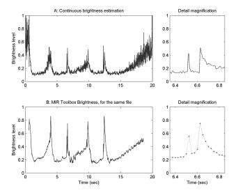
**Fig. 5.** The same sound of Fig. 2 analyzed with CoBE and with MIR Toolbox Brightness: As shown in the right side of the plot CoBE can obtain finer temporal precision because it does not rely on signal framing.
