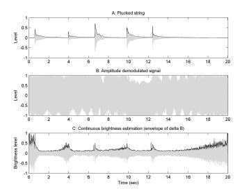
**Fig. 2.** A: Input signal. We recorded a plucked instrument with some background noise coming from the amplifier; B: Input divided by its amplitude envelope; C: Filtered version of B, showing the percentage of the input matching the filter characteristic. Brightness increases when the notes fades out due to the presence of noise.
