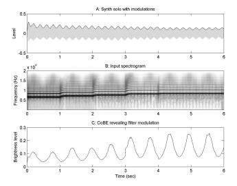
Fig. 3. Due to the HPF, high frequencies have a great influence over brightness estimation, this can help revealing lowpass filter modulations despite of amplitude and pitch changes.
