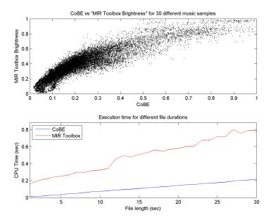
**Fig. 6.** (upper) Plotting the results of 30 different music samples, analyzed with CoBE and with MIR Toolbox Brightness. (lower) Execution time for different samples length. The computational cost for CoBE seems to be of a lower order of complexity.
