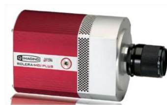
Figure 8: (Top) Image of CCD camera used to detect the fluorescence of the single Cy3 molecules.. (40)
