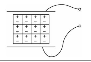
Figure 2.5 Generic example of a piezoelectric transducer. Mechanical force will distort the alignment of the dipoles forming an electric current between the electrodes.
