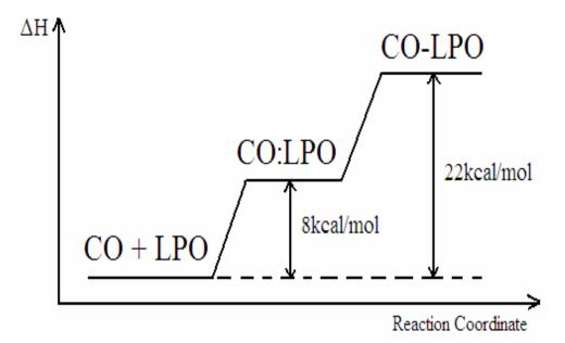
Figure 4.2: Enthalpy profile of CO binding to LPO
