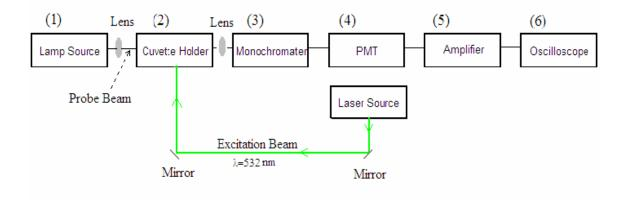
Figure 2.2: Instrumentation set-up for transient absorption spectroscopy.
