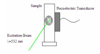
Figure 2.4 Acoustic wave generated in sample by laser pulse excitation beam.
