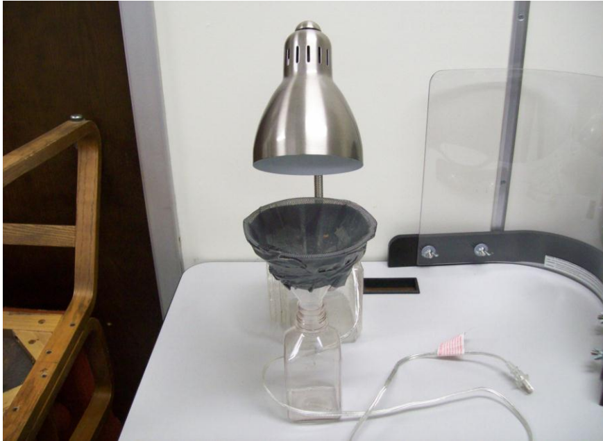
Figure 9: Example of Berlese set-up in lab; soil would go on mesh and the container below would be filled with alcohol for arthropod preservation (Source: Taylor Brewer, 2011).
