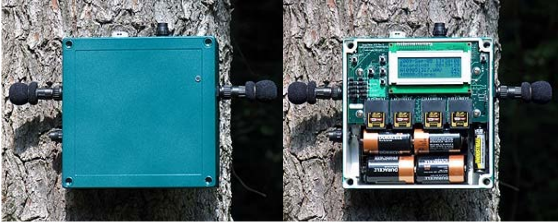
Figure 21: A Song Meter SM2™ automated digital recording device, designed by Wildlife Acoustics, attached to a tree. The left image has the cover on, and the right image is with the cover removed, revealing the controls. Photo courtesy of Wildlife Acoustics.
