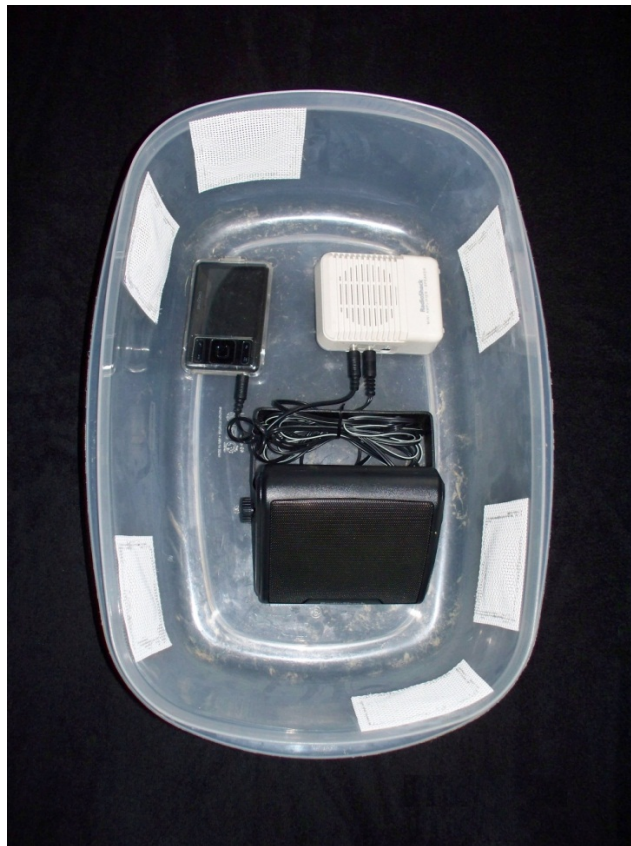
Figure 22: The ‘callbox’ used to play breeding calls during experimental surveys. In the top left of the plastic storage bin is the MP3 player, which is attached to the amplifier on the top right. That is wired to the loudspeaker in the bottom of the box. The holes covered with plastic meshing on the sides allow sound to clearly escape the box. In the field, it would also have an airtight lid covering it.
