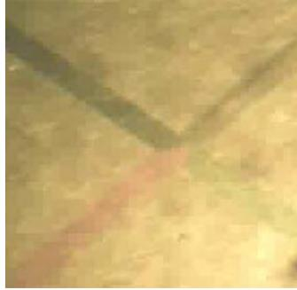
**Figure 19.** Laminar flow in microfluidic channels containing blue (top left), red (bottom left), and green (bottom right) dye solutions. The dyes enter through input channels, meet at the intersection, and display laminar flow in the output channel. Three parallel flows can be seen in the output channel since mixing of the dyes does not occur.
