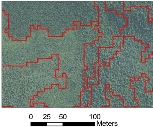
**Figure 7: Object oriented segmentation of Landsat image overlaid on NAIP imagery. Image zoomed in to show size and texture.**
