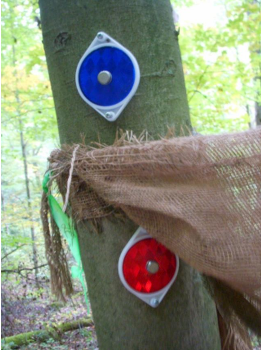
Figure 26. Photo of data logger set up. Each site had 1 data logger placed on a tree to collect ambient temperature and relative humidity. I placed 1 data logger under burlap on the same tree to collect temperature and relative humidity under burlap.
