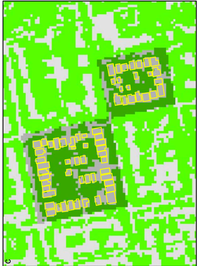
Figure 6. Classified NDVI image to show the areas covered by sealed surfaces or vegetation for the Hal Greer study areas. Building footprints are given to show which sealed surfaces are roofs. a) HG1. b) HG2. c) HG3 in the upper left and HG4 in the lower right.
