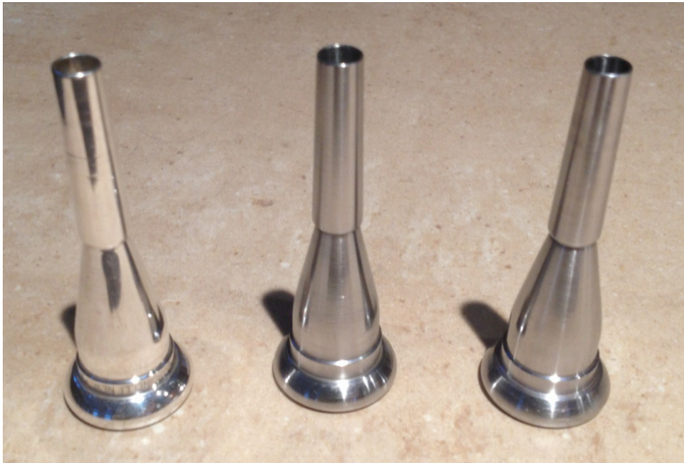
Figure 8 - (left to right) Original, steel, cast iron
