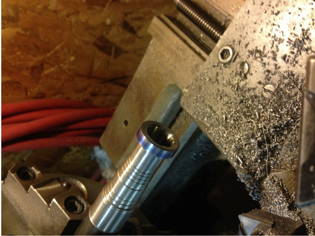
Finishing turning shoulder behind rim to final diameter
