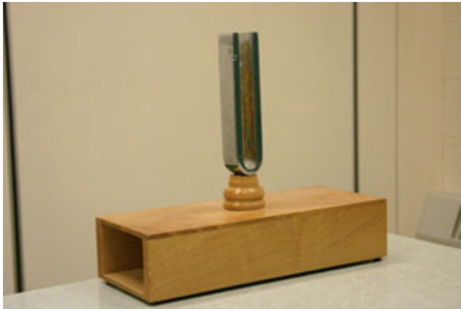
Figure 2 - Tuning fork attached to a wooden box illustrating resonance
