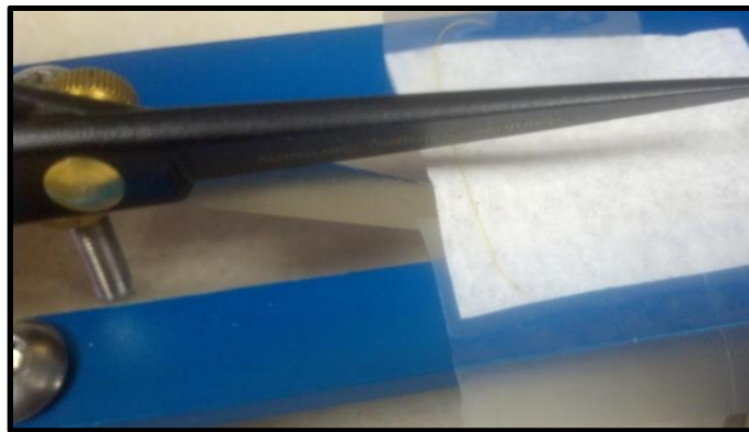
Figure 2. Scissors Test. Bamboo fibers are affixed to a paper towel when cutting to prevent the fiber from moving during the cut. Both leaves and paper towels are anchored to the stage by tape to prevent movement. Caution must be taken during taping to ensure no tape is in the path of the scissor blades.
