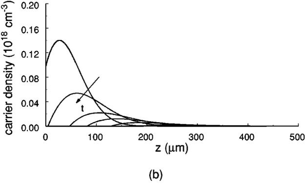
FIG. 2. Time-dependent evolution of the carrier density profile in Si after UV excitation for nonconstant transport parameters and  $S=10^3$  cm/s. (a) Six equidistant time steps from 1 to 6 ns. (b) Six equidistant time steps from 1 to 6  $\mu\text{m}$ .
