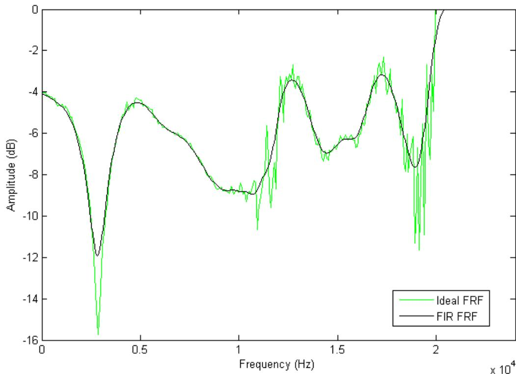
**FIGURE 3:** Comparison between measured on-axis frequency response of the ear canal and its FIR reproduction
