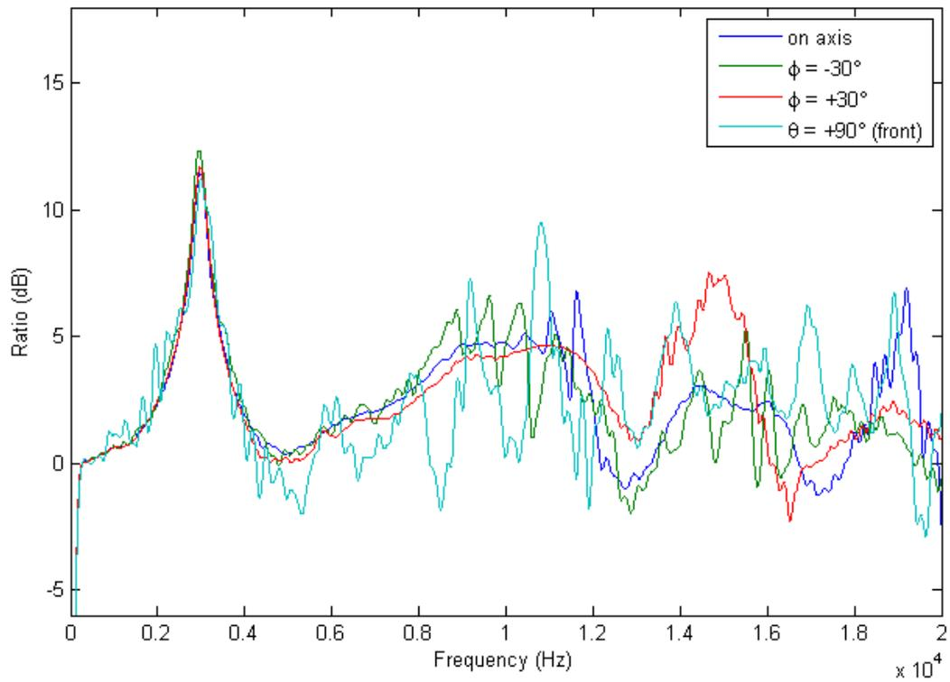
FIGURE 2: Calculated ear canal frequency responses for different positions along azimuth and elevation coordinates.
