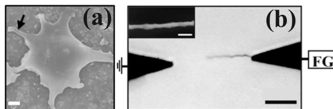
FIG. 1. (a) Scanning electron micrograph of fixed *D. discoideum* cell with extending pseudopods. Scale bar = 1  $\mu\text{m}$ . (b) Optical micrograph of PEDOT filament grown by the DNA technique. FG  $\equiv$  function generator. Scale bar = 10  $\mu\text{m}$ . Inset: a scanning electron micrograph of a filament. Scale bar = 1  $\mu\text{m}$ .
