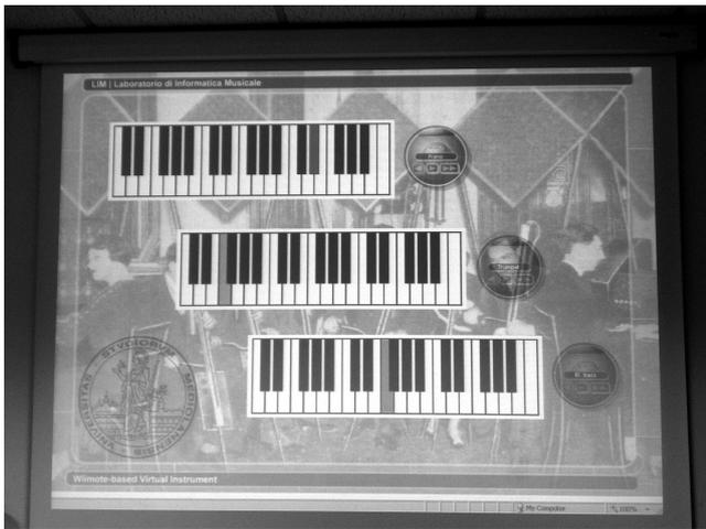
**Figure 1: The multi-keyboard interface projected onto a wall. Pressed keys are colored: the main color represents the association with a controller, whereas the brightness is related to key velocity.**
