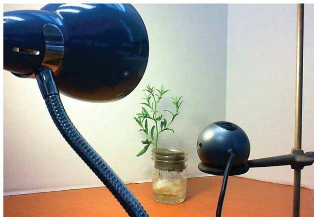
FIGURE 1. A simple webcam set-up using a white tri-fold poster board. In this set-up, a Logitech QuickCam is mounted on a ring attached to a ring stand.
