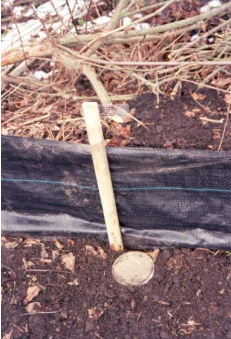
Figure 2.2 Drift fence with covered pitfall trap at Boaz Swamp.
