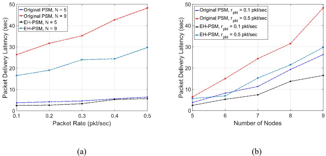
**Figure 7. The performance of packet transmission latency against packet rate and number of nodes.**
