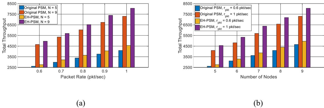
**Figure 6. The performance of throughput against packet rate and number of nodes.**
