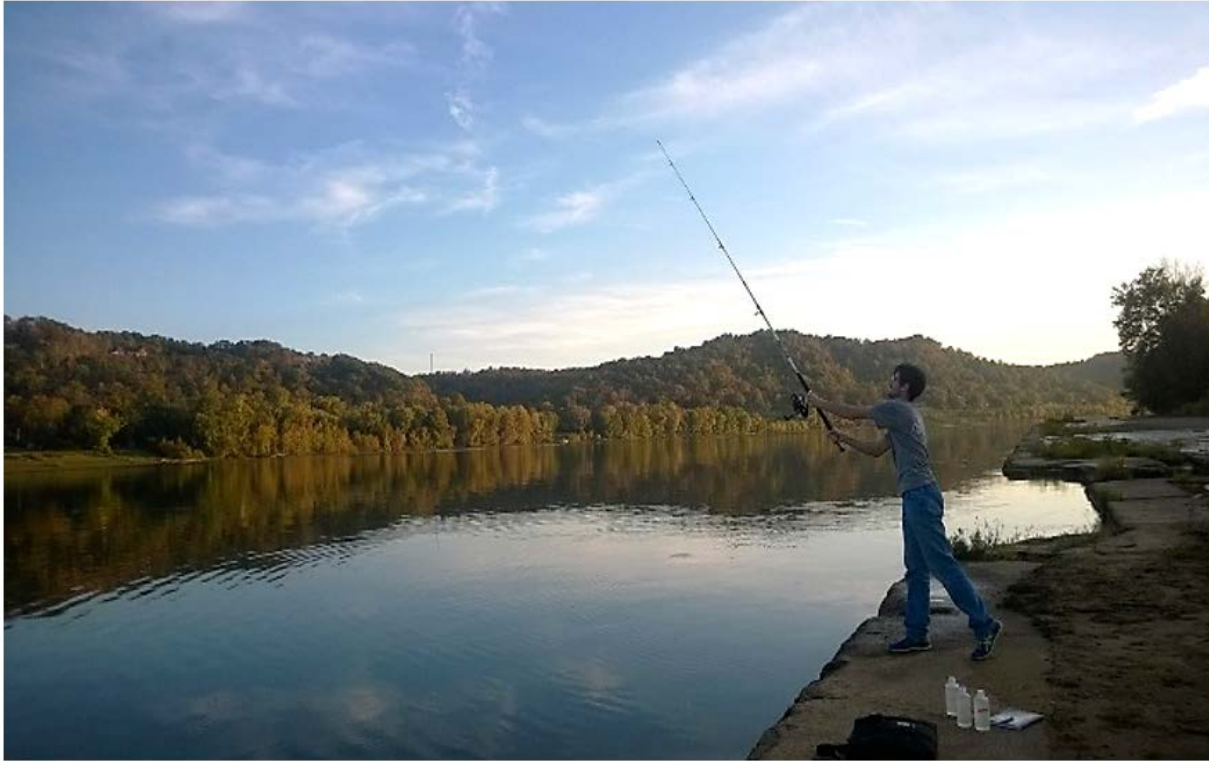
Figure 4. A 500 mL Nalgene bottle was attached to the end of a fishing pole and cast into the Ohio River to obtain samples away from shore not using a boat.
