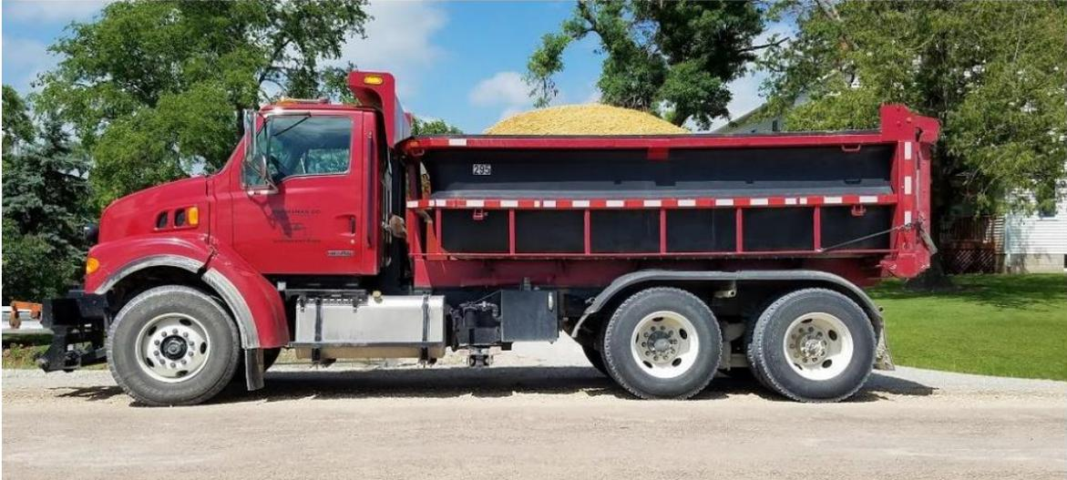
*Figure 16: Tandem-Axle Dump Truck (Gibbs, 2017)*
