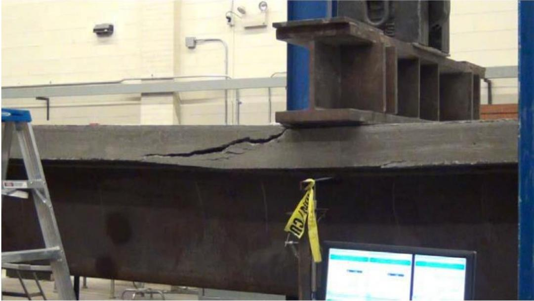
***Figure 6: Typical Failure mode for Composite Specimens (Michaelson, 2014)***
