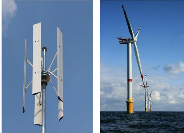
**Figure 4.** The two main designs of wind turbines: vertical axis wind turbine (left), and horizontal axis turbine (right).
