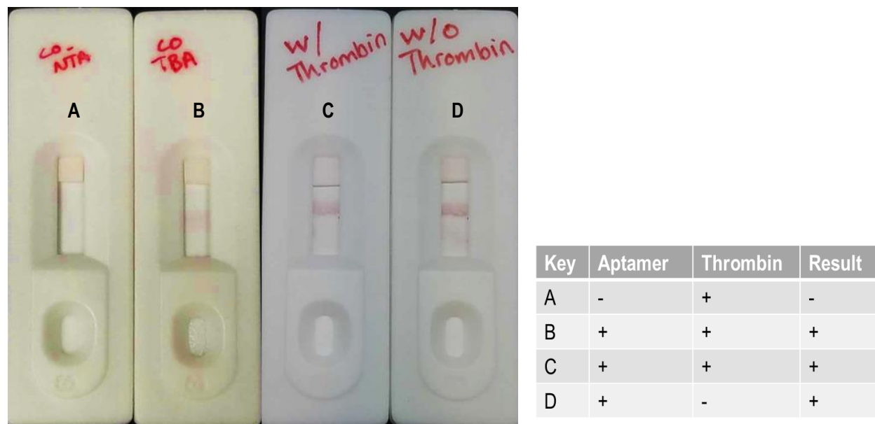
Figure 47 – Image of CO_TBA based LFA control experiment. Negative (A and D) and positive (B and C) control TBA LFA experiments. Successful sandwich-style capture can be seen in the positive control assay. The negative control assay which has no thrombin-binding aptamers on the immobile probe did not show a signal. Right image: Both LFAs showing capture means that thrombin-binding aptamers TBA29 and TBA15 bind to each other and give a signal.
