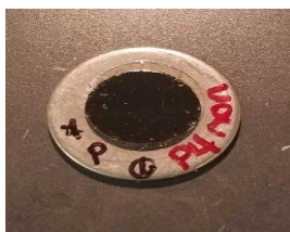
Figure 13 - Mica disc for AFM imaging. Prepared mica slip used for sample deposition and visualization using AFM.
