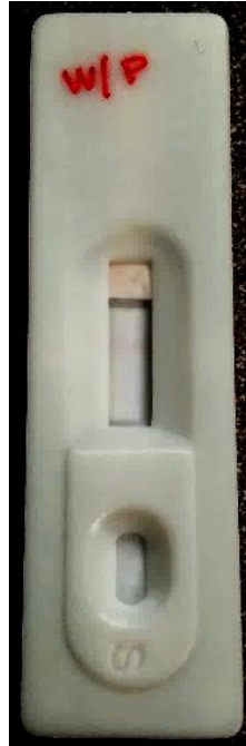
Figure 49 – Version 2 of CO_TBA(M) LFA. Version 2 of CO_TBA(M) tested against Thrombin immobilized onto the NC membrane. Positive capture displayed by the test.
