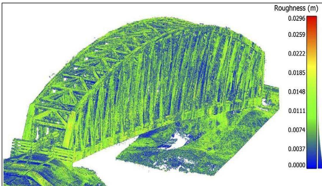
**Figure 29: Example of Hierarchical Point Cloud Generation (HPCG) based 3D point cloud generation.**
