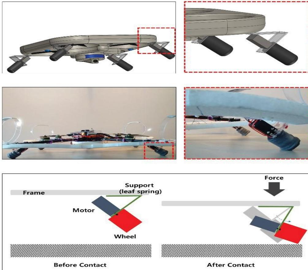
**Figure 23: Wall-sticking and climbing robot UAV prototype.**
