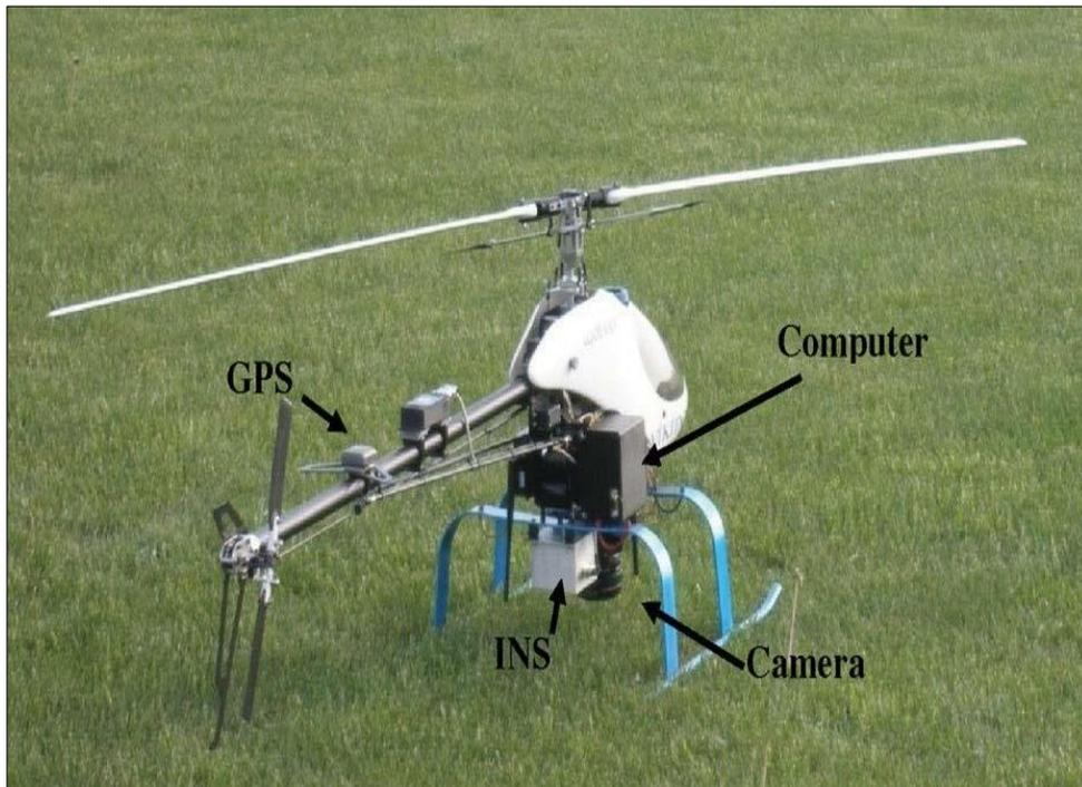
**Figure 10: Example of a single rotor UAV**
