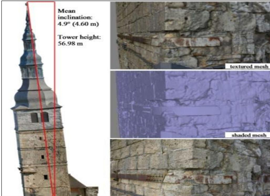
**Figure 17: Angular displacement detection in tall structure, right: 3D construction model using dense point cloud method.**
