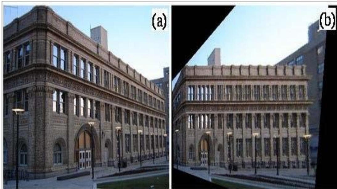
**Figure 22: Image flattening technique (a) original image (b) flattened image with MatLab algorithms.**
