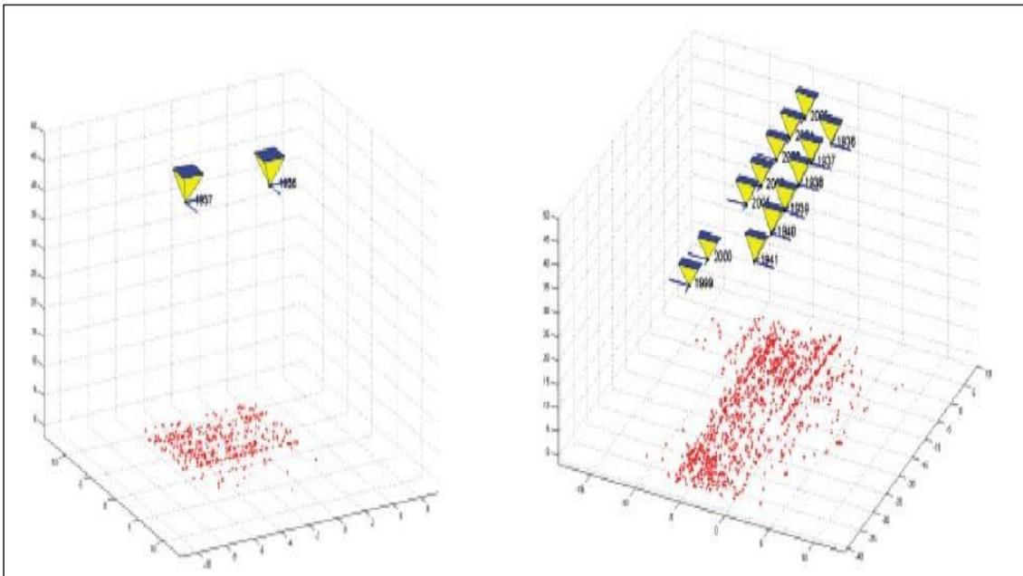
**Figure 19: 3D block formation and point generation. Inverted pyramids represent the camera position and the red points represent the spatial position of the object under analysis.**
