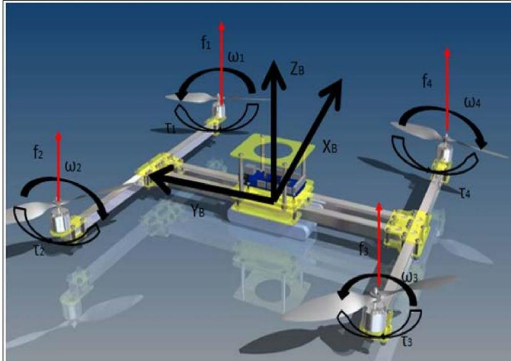
**Figure 20: Proposed prototype design for the application of vector thrust mechanism.** The figure is referenced from Kuo et al. [20].
