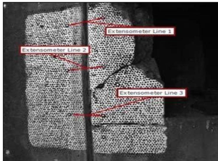
**Figure 18: Displacement detection in the expansion joint.**
