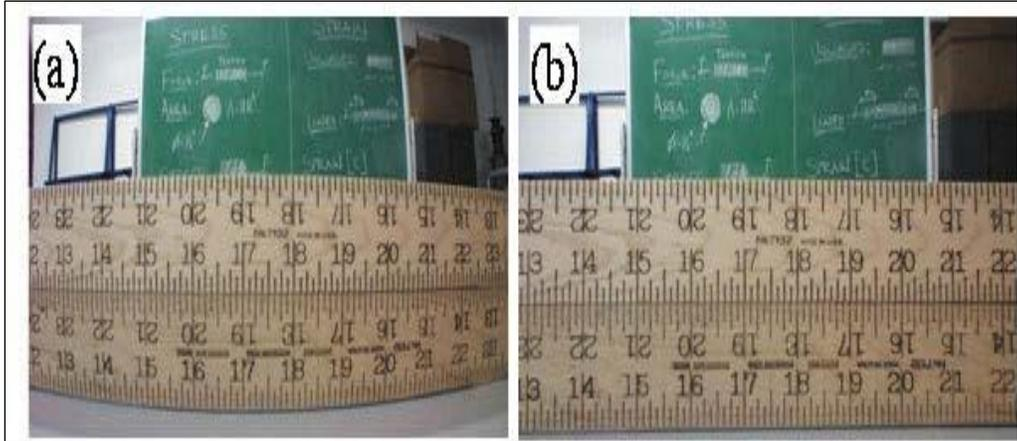
**Figure 21: Lens distortion correction (a) image with distortion (b) corrected image with MatLab algorithms**
