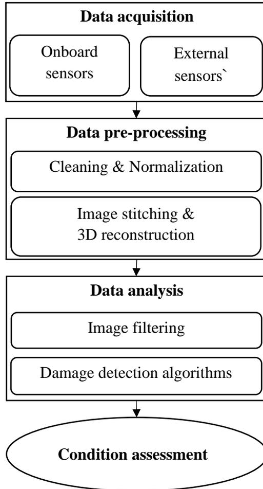
**Figure 24: UAV assisted SHM workflow**
