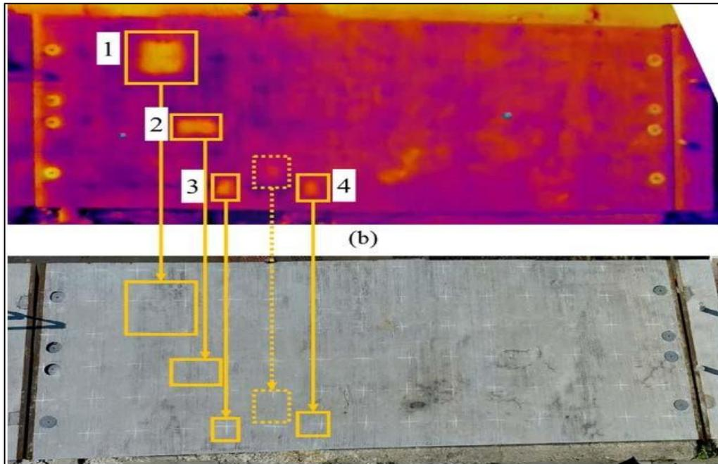
**Figure 15: UAV infrared images (a) used for delamination detection and UAV color images (b) stitched together.**
