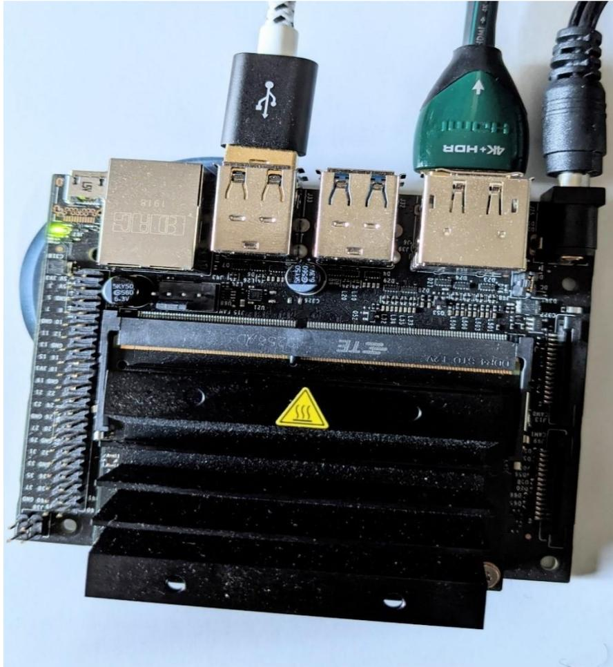
**Figure 37: Nvidia Jetson Nano as Edge Computing Platform**
