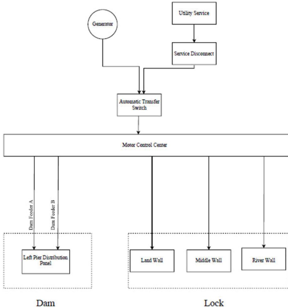
**Figure 6- Lock and Dam System Overview**
