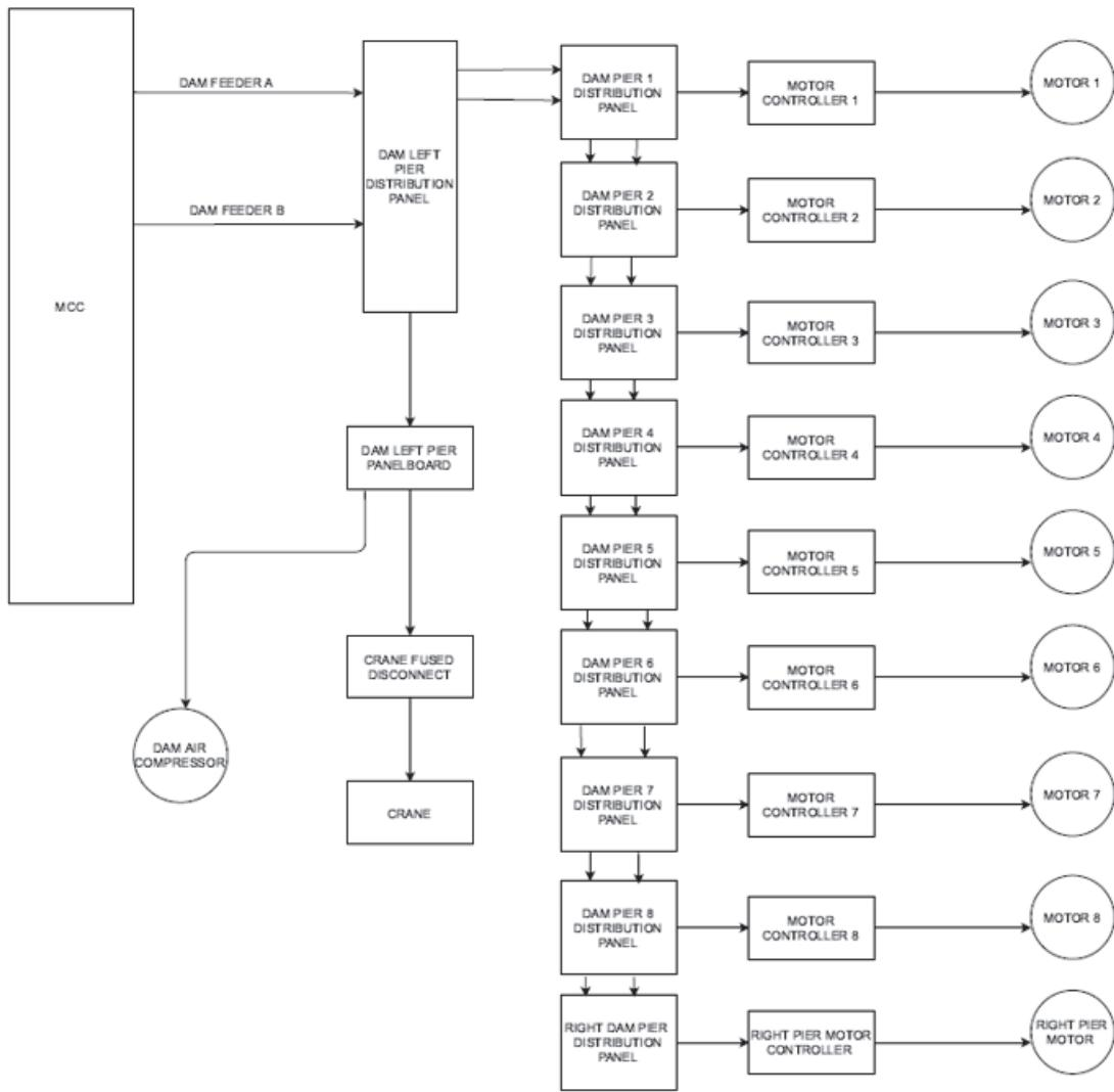
**Figure 7- Lock and Dam-Dam**
