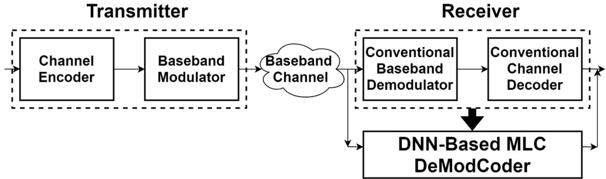
**Figure 5. A Point-to-Point Communication Link with Conventional vs. AI Based Receiver Processing.**
