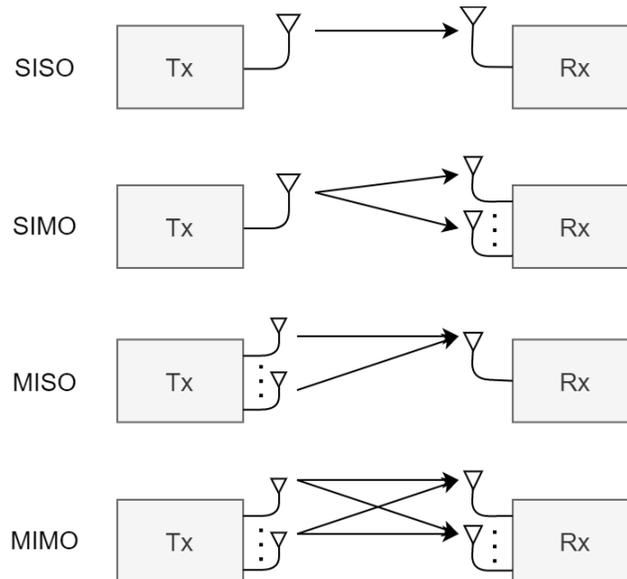
**Figure 3. System Structures of SISO, SIMO, MISO, and MIMO.**
