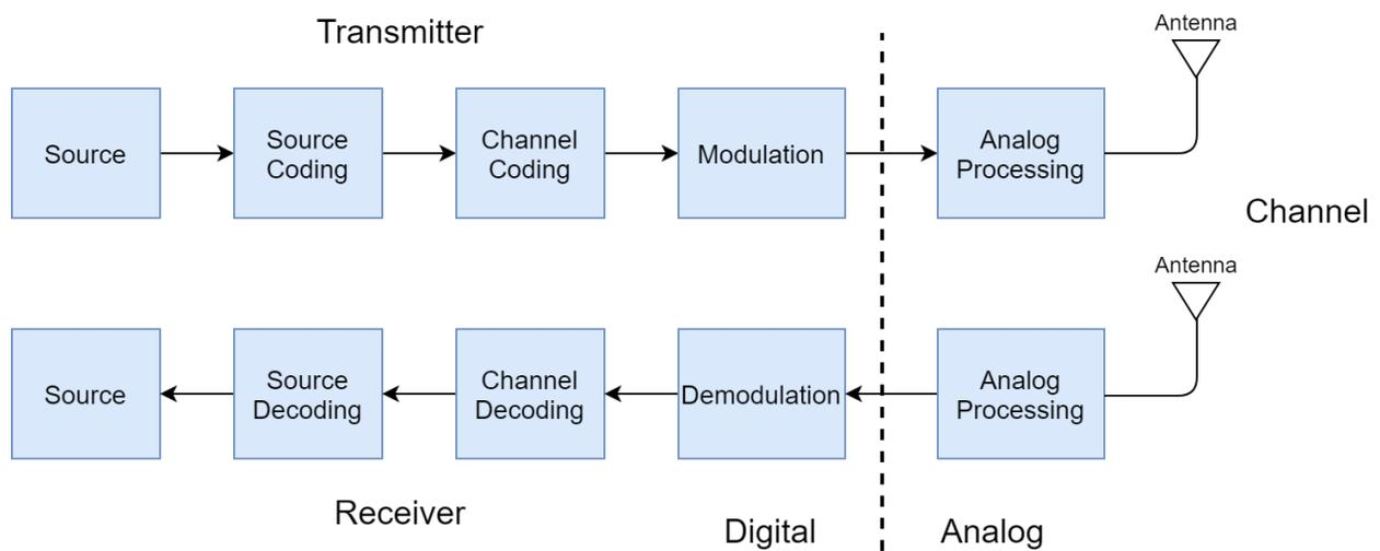
**Figure 1. Block Diagram of Digital Communication System.**
