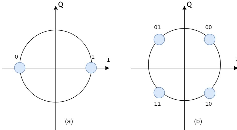
**Figure 2. Constellation Diagram of (a) BPSK and (b) 4-QAM.**
