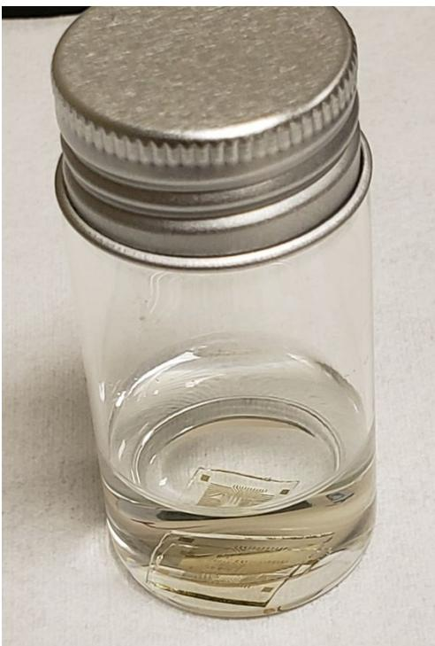
**Fig. 8. DEP chip in solution**
