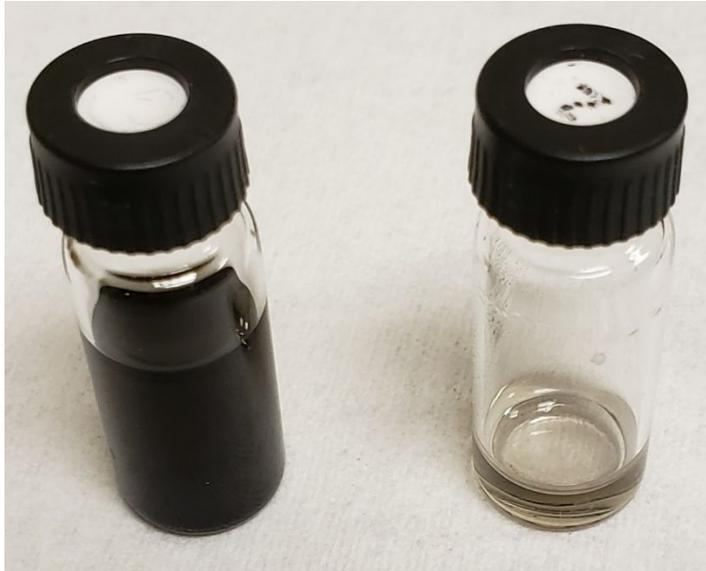
**Fig. 9. Carbon nanotube solution versus the working solution**
