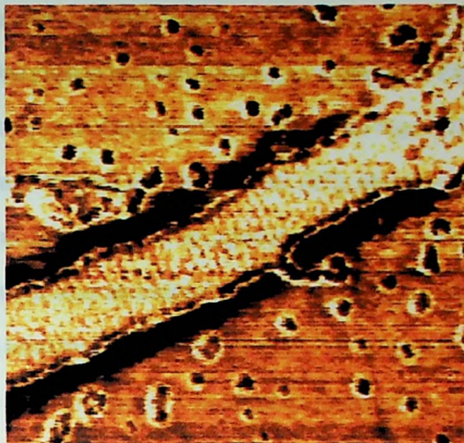
Figure 20: Phase image of 1.351 \mu\text{m} view of DNA nanoarray seen in Figure 12.
