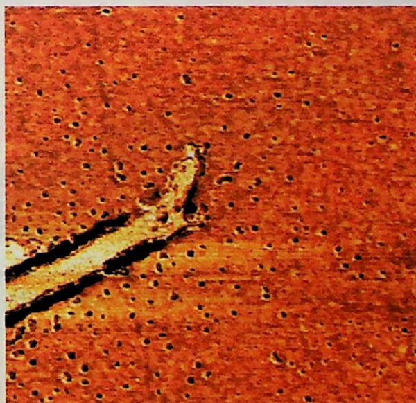
Figure 19: Flattened phase image of tip of DNA nanoarray. The black dots surrounding the array are believed to be DNA fragments. Scan size 3.271\mu\text{m} .
