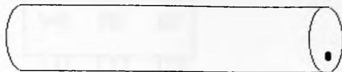
Fig. 8, Teflon holder for large cell.
