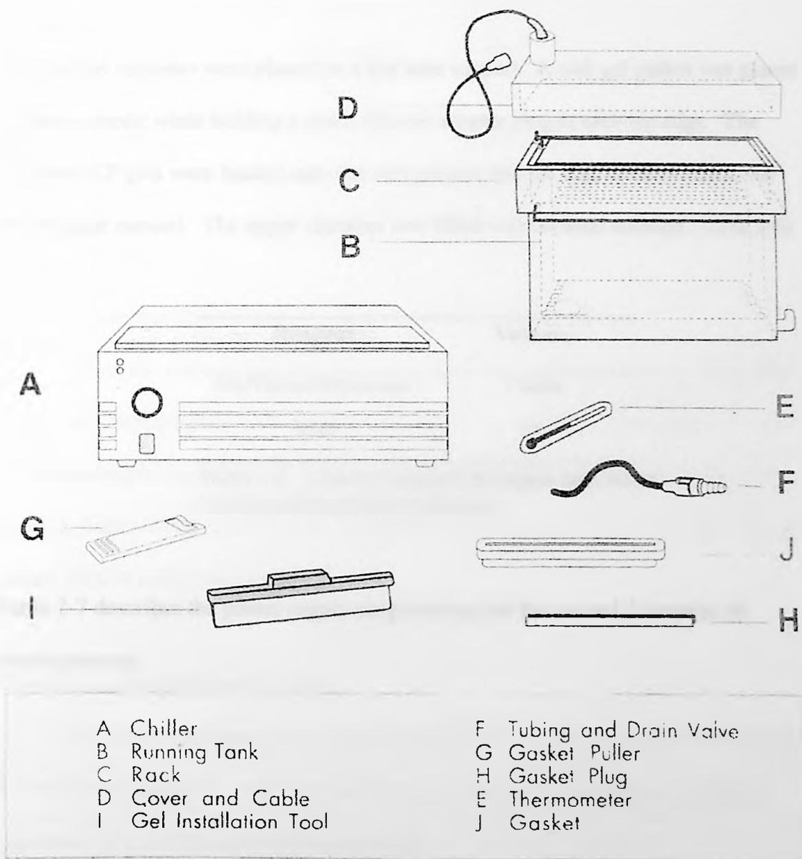
Figure 2-6. Components of the Investigator 2-D running system used for slab gel electrophoresis.<sup>24</sup>
