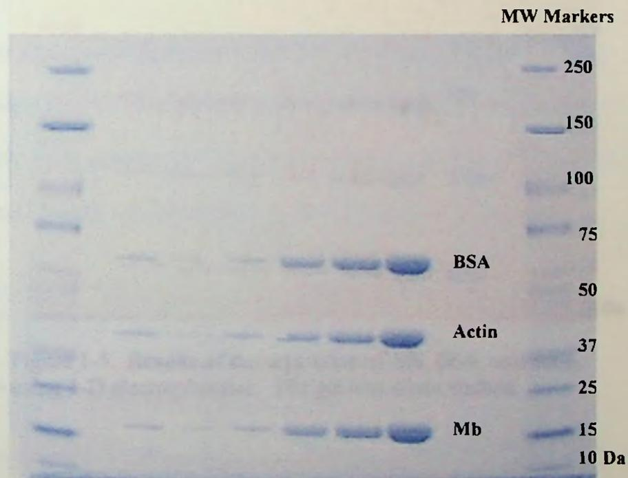
Figure 1-4. Results of the separation of Mb, BSA, and actin using 1-D electrophoresis. Gel was stained with Coomassie.
