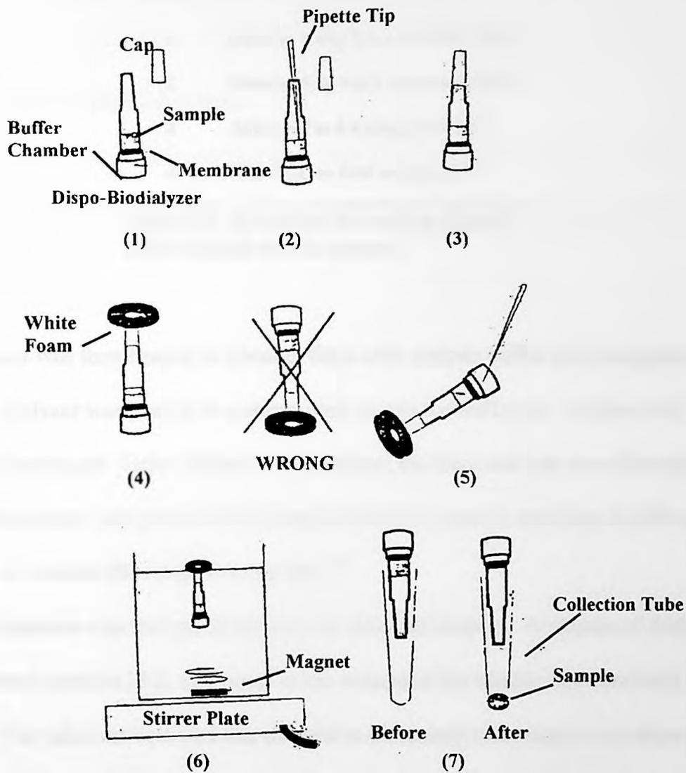
Figure 2-7. Procedure for using the Bio-dialyzer to perform dialysis on samples.<sup>25</sup>
