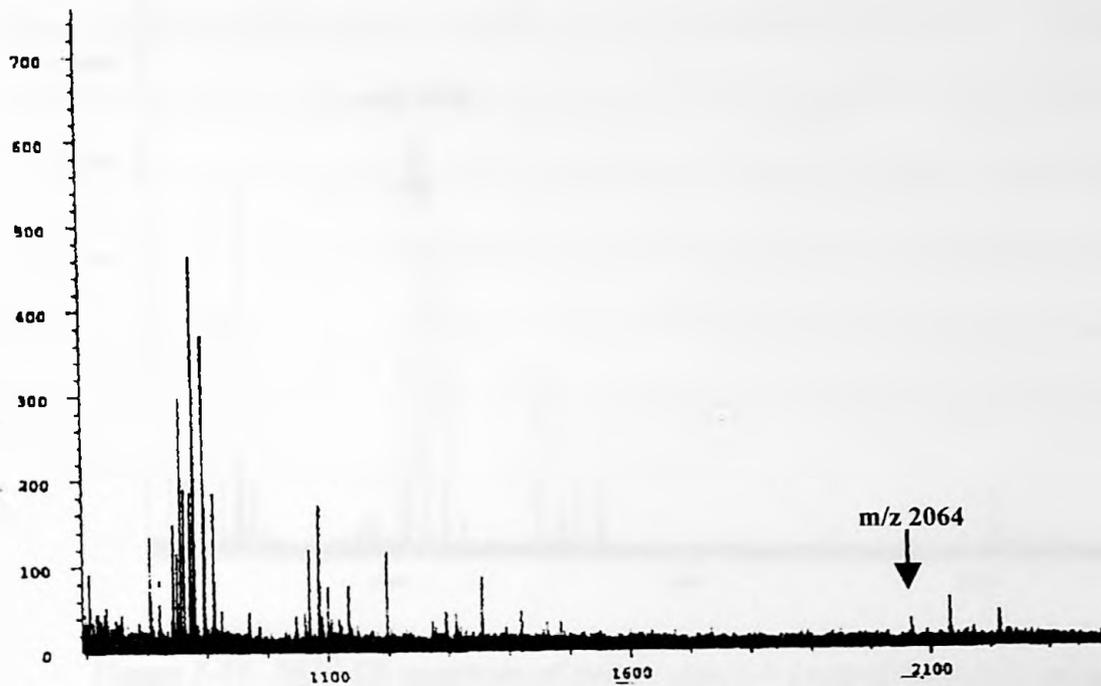
Figure 2-18. MALDI spectrum of proapo A-I excised from 2-D gel and digested using trypsin.
