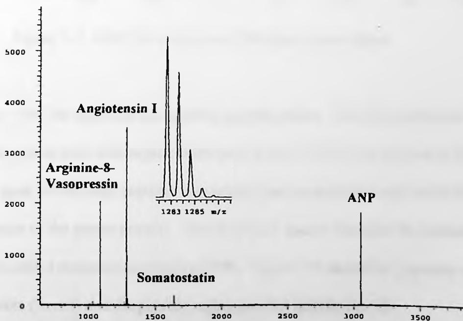
Figure 1-6. MALDI spectrum of the peptide standard used to calibrate the instrument.
