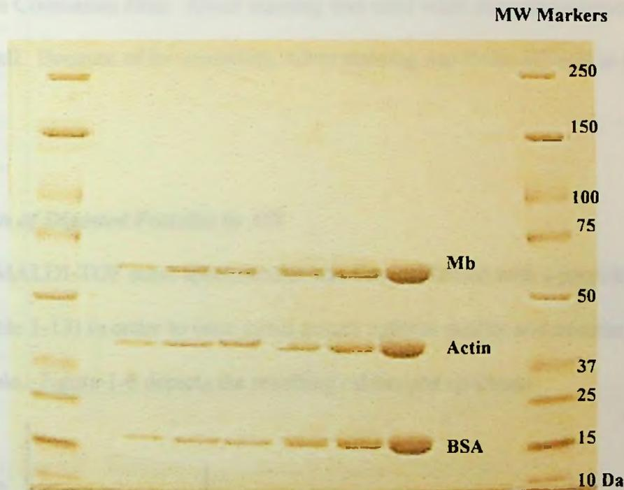
Figure 1-5. Results of the separation of Mb, BSA, and actin using 1-D electrophoresis. The gel was silver stained.
