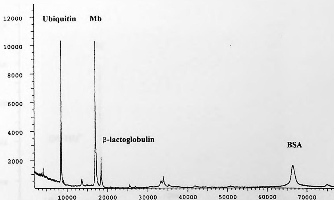
Figure 1-2. MALDI spectrum of a protein standard used for calibration of the instrument.
