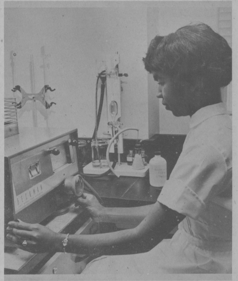
MARGIE COBBS, Huntington Sr., is shown working at the Flame Photometer, which determines the amount of sodium or potassium in blood serum. Margie is presently doing work in the Electrocardiograph, Basal Metabolism department.
