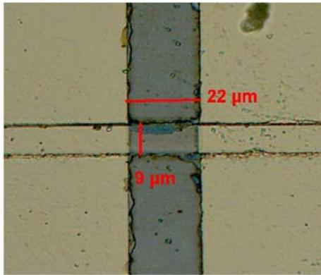
**Figure 1.** Optical micrograph of a portion of the microbolometer.
