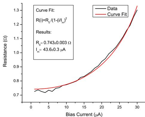
**Figure 2.** (color online) Curve fit as per [1] to obtain the bolometer's characteristic current  $I_m = 43.6 \mu\text{A}$  at 1.759 K.
