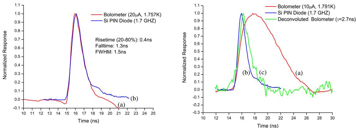
**Figure 3.** (color online) *Left:* Bolometer (a) and Si PIN diode (b) responses to same photoexcitation. Bias current 20  $\mu\text{A}$ ,  $T=1.757$ . Note:  $\tau < 0.74$  ns. *Right:* bolometer (a), Si PIN diode (b), and deconvoluted bolometer (c) responses to same photoexcitation. Bias current 10  $\mu\text{A}$ ,  $T=1.791$  K. Note  $\tau=2.7$  ns
