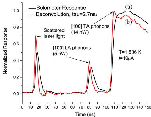
**Figure 4.** (color online) Normalized bolometer response (a) and deconvoluted absorbed power (b) in a heat pulse experiment. Note: Upon deconvolution TA phonon arrival can be clearly resolved and ballistic LA and TA time-of-flights agree (to 1%) with those expected for a 0.544 mm thick substrate; the phonon pulse widths are comparable to the laser pulse excitation. Phonon focusing accounts for the increased TA peak height and a diffusive TA tail is observed.
