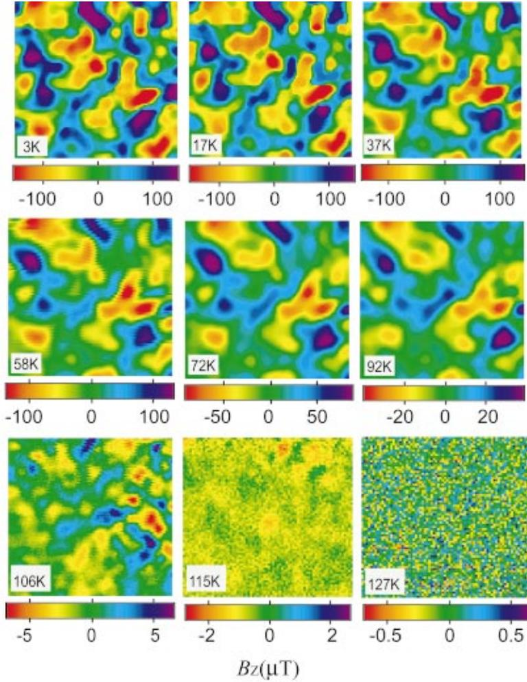
FIG. 2. (Color) Scanning SQUID images of  $\text{Nd}_{0.7}\text{Ca}_{0.3}\text{MnO}_3$  single crystal at different temperatures. The image sizes are  $800 \mu\text{m} \times 800 \mu\text{m}$ . The color bars indicate the  $B_z$  scales in units of  $\mu\text{T}$ .
