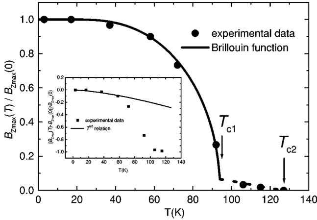
FIG. 3. Maximum field  $B_{zmax}$  obtained from the scanning SQUID image as a function of temperature. The solid line denotes the Brillouin function with  $T_c = 95$  K. The dotted line is a guide for the eye for the experimental data at  $T_{c1} \leq T \leq T_{c2}$ . The inset shows Bloch's  $T^{3/2}$  function fitted to the experimental  $B_{zmax}$  below 60 K.
