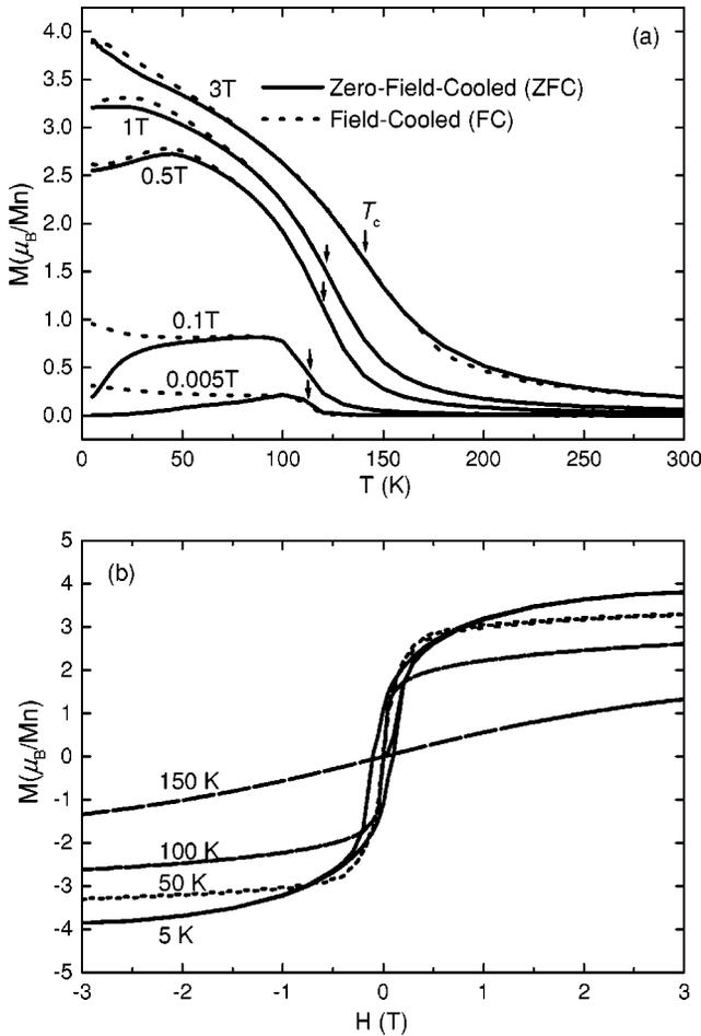
FIG. 1. (a) Zero-field-cooled (ZFC) and field-cooled (FC) magnetization as a function of temperature at different fields.  $T_c$  is indicated by arrows. (b) Field dependence of the magnetization at different temperatures.
